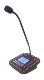
Fully monitored desk call station according to EN54-16. 10 keys dial keyboard, "Talk" and "Clear" key, 3 Evac activation keys, touch screen quarter VGA TFT display, dynamic gooseneck microphone, DSP audio processing. All keys and functions are software programmable. Wiring by Rj45 connector and CAT5 Cable. Power supply from RJ45 cable or 24Vdc local adaptor.
