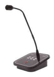
Fully monitored desk call station according to **EN54-16**. Software programmable capacitive selection keys, "Talk" and "Busy" Keys, "System" LEDs, dynamic gooseneck microphone, automatic compressor, level adjustment trimmer. Wiring by RJ45 connector and CAT5 Cable. Wiring by RJ45 connector and CAT5 Cable.
