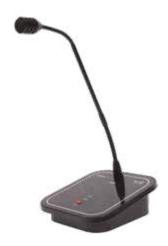
Fully monitored desk call station according to **EN54-16**. Software programmable "Talk" key, "Busy" and "System" LEDs, dynamic gooseneck microphone, automatic compressor, level adjustment trimmer Wiring by Rj45 connector and CAT5 Cable.
