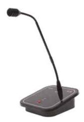
Fully monitored desk call station according to EN54-16. Software programmable "Talk" key, "Busy" and "System" LEDs, dynamic gooseneck microphone, automatic compressor, level adjustment trimmer Wiring by Rj45 connector and CAT5 Cable. Power supply from RJ45 cable or 24Vdc local adaptor.
